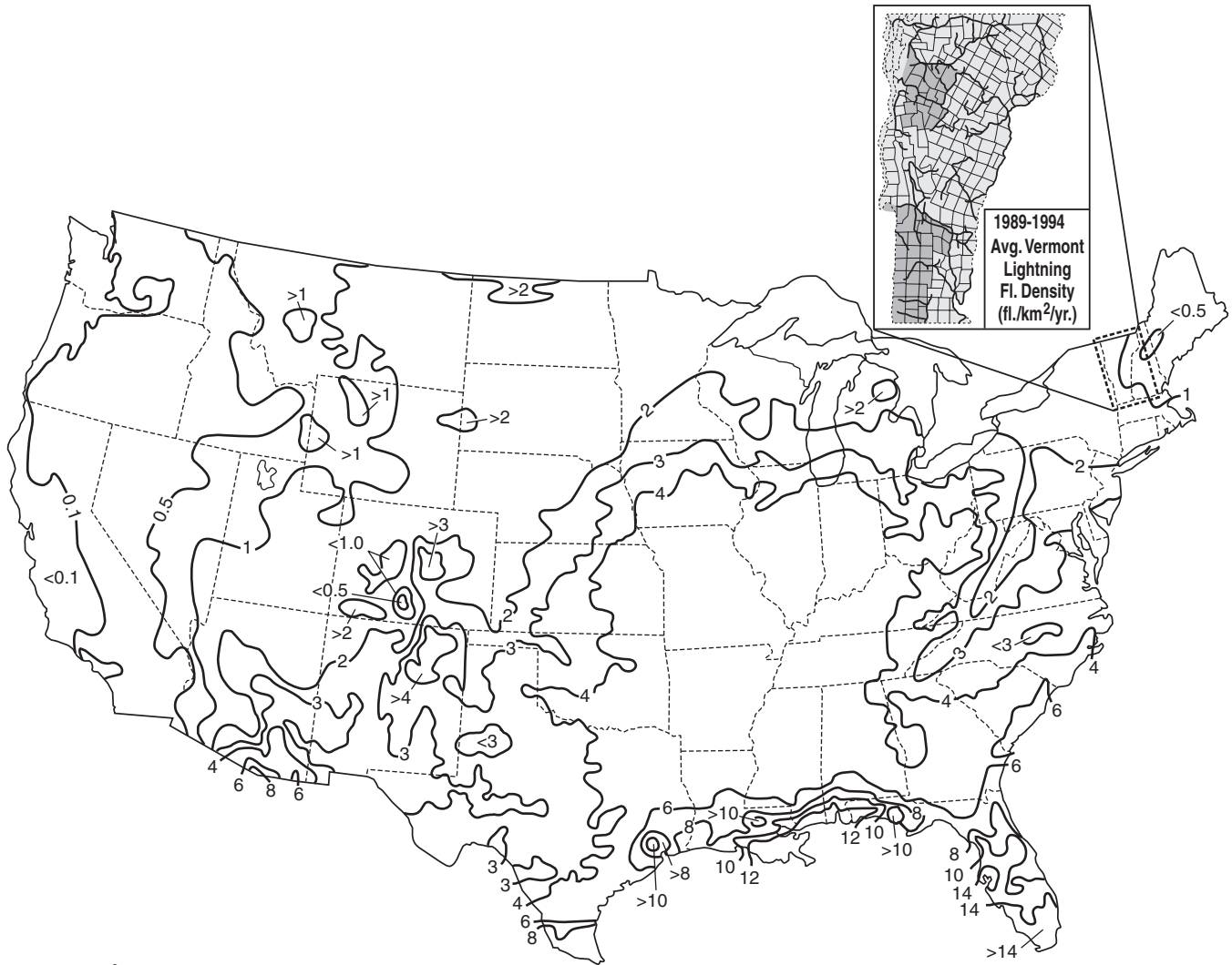
FIGURE H.2 1989–1998 average U.S. lightning flash density in flashes/km 2 /year. (Courtesy Global Atmospheric, Inc.)
