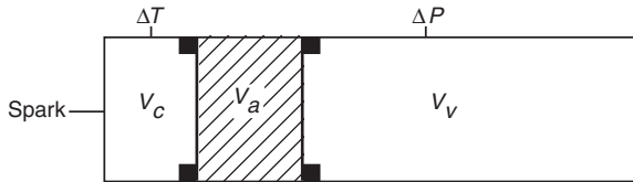
FIGURE A.14.3.7 Double Void Explosion Suppression Test Setup (MIL-PRF-87260B).
