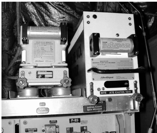
FIGURE 13.5(a) Flight Data Recorder and Cockpit Voice Recorder.
