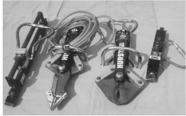
FIGURE 9.4.3(d) Hydraulic Rescue Tools [from left: life or spread (long), spread cut, and lift or spread (short)].
