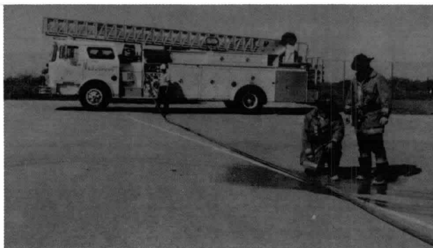
Figure A-8-4.2.7 Pressure test layout with inspection personnel checking couplings. (Courtesy of Rockford, Illinois Fire Department)
