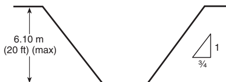
FIGURE B.1.1.1(a) Simple Slope — General. [Source: 29 CFR 1926, Subpart P, Appendix B, Figure B-1.1.1(a)]
