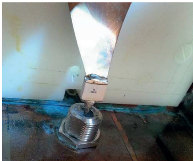
Figure C.3 — Matching capacitor connection
