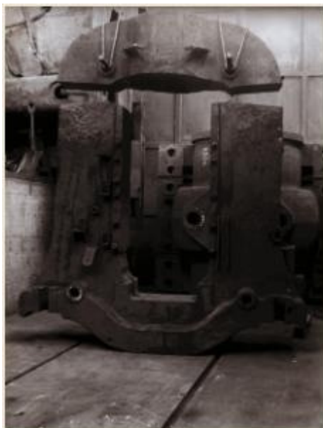
Figure 37 — Screw press column before repair welding
