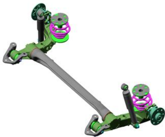
Figure 24 — Magnetarc-welded rear axle
