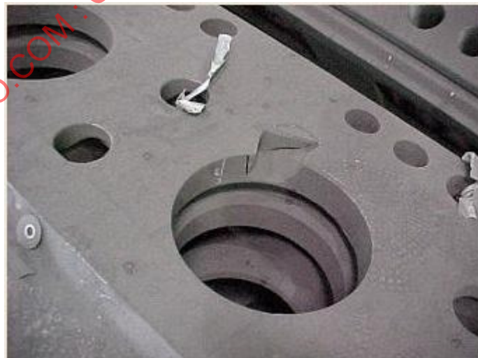
Figure 30 — Defective spot detected by ultrasonic testing after blast cleaning and after first-process machining
