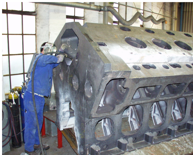
Figure 11 — Finishing welding at the 18-cylinder engine block
