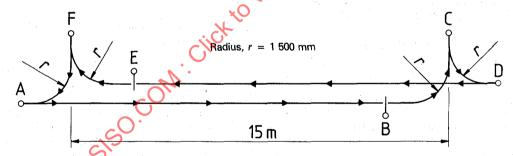
Start and end each cycle at A Employ maximum acceleration and retardation when changing speed.
