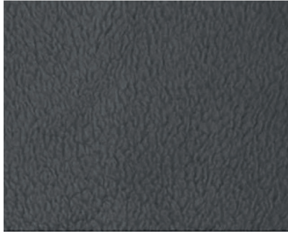
Figure 1 — Example of matting appearance of napped fabric
