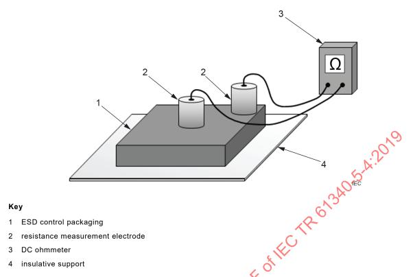
Figure 18 - Setup for test method using two resistance measurement electrodes
