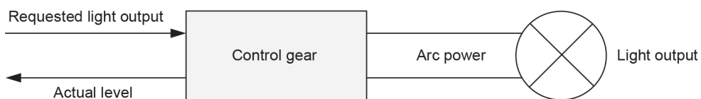
Figure 2 – Control gear directly operating a light source
