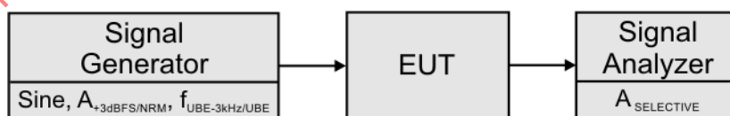
Figure 27 – Non-linear cross-talk method
