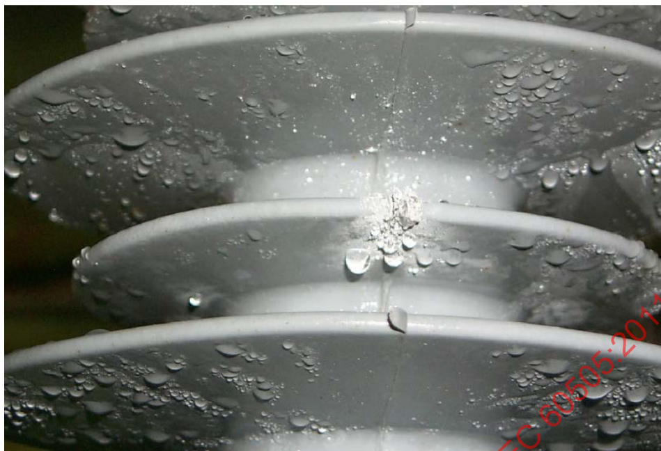
Figure A.37 – After 11 years in service UV and moisture impact
