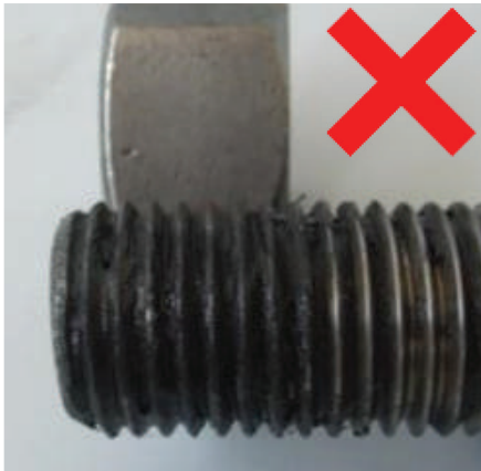
(a) Insufficient Lubrication: Lack of Fill Between Root and Crest of Threads
